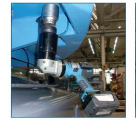
Accuracy and consistency. Built to a high standard of precision, to ensure accurate torque application, every time, reducing the risk of over or under tightening
