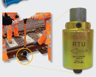
Modification of RTU for Track Bolt Tightening
