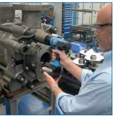
This increases the running time of the battery and maintains the torque at a constant level. This allows the tightening torque for each bolting operation to be precisely maintained and ensures stable torque accuracy over the entire discharging cycle of the battery
