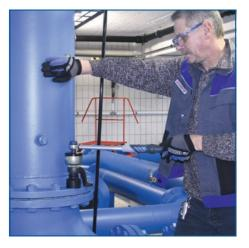
Overload safety. An integrated overload safety mechanism protects the gear unit, by ensuring that the square drive has a pre-determined breaking point. The square shears if overloaded and is easily replaced
