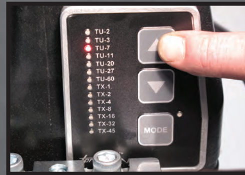
PUSH BUTTON TOOL SELECTION FOR TORCUP TU AND TX WRENCHES
